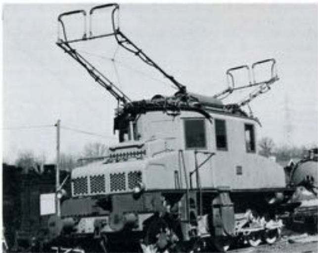
FERROVIE DELLA STATO (Italian State Railways): Built around 1910 by an Italian subsidiary of Westinghouse, this freight locomotive operated off a three-phase, 3,000-volt A.C. electrical system and developed 2,000 horsepower from its two motors. It had a top speed of 31 mph. The engine arrived at NMOT in 1968.
